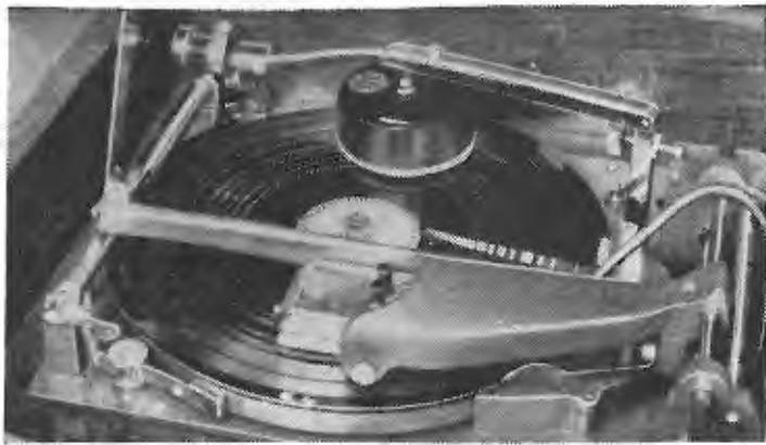
Recorder unit used in the M.S.S. radio-gramophone showing the new "Rotacol" swarf collector.
