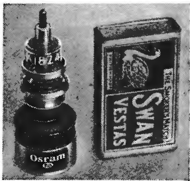
G.E.C. disc-seal transmitting tetrode with forced air cooled anode.
